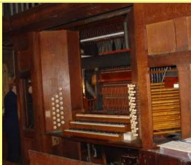
The three keyboards, and connecting rods for all the various organ stops are seen here, all linked up and ready to command musical sounds again.
